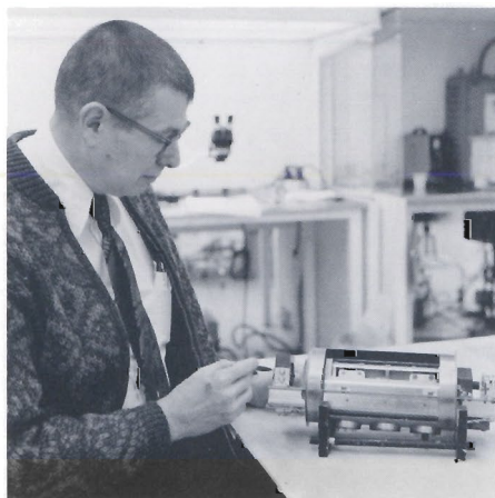
The heart of an HP cesium beam standard—"atomic clock"—was explained by physicist Len Cutler of HP Labs in 1977 photo.
